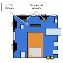
Configure the jumpers wires on the TTL level header as indicated in the image above and the table below
