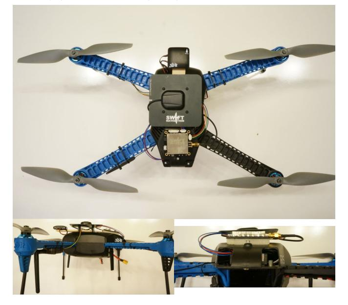
RTK GPS provides a "pseudo-absolute" position: a centimeter-accurate position relative to the arbitrarily-accurate ground station positon. Many applications don't require an extremely accurate ground station location, caring only about positioning *relative* to a known fixed point. For example, accurate landings and takeoffs, or logging accurate relative locations of pictures.
